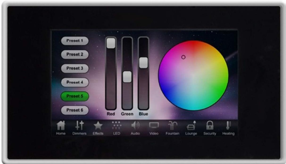
The complete installation, meaning basic and ambient lighting, as well as the media application is controlled via a digital glass touch RGB LED user interface.
